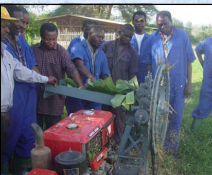
Utilization of hand tractor power for chopping grass and other animal feeds.
